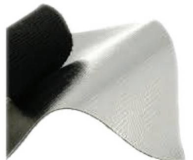
Peel: Pass (ASTM D903) | Tensile: Pass (ASTM D5035) | Tear: Pass (ASTM D1938)
